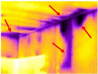
This image shows a significant difference and inconsistent distribution in colour / temperatures which would indicate the presence of a thermal anomaly and would require further investigation.
